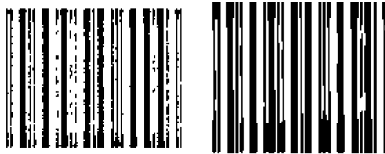
Fig. 2. In the left image, a degraded barcode due to the use of regional thresholding is shown. In the right image, the result of reconstruction of the same barcode using morphological dilatation is shown.
